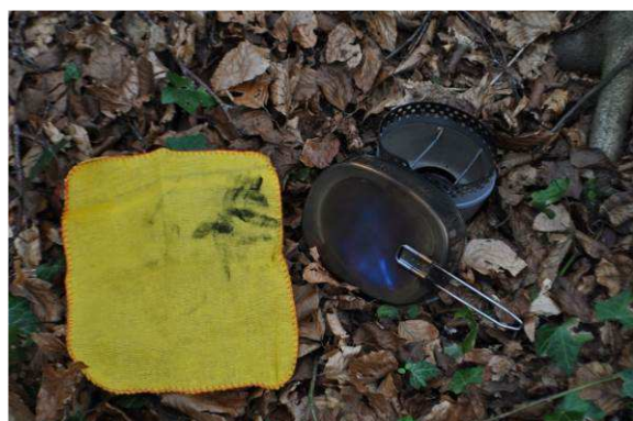
FireDragon – Soot removed from base of cooker after burning 1 block of fuel.
