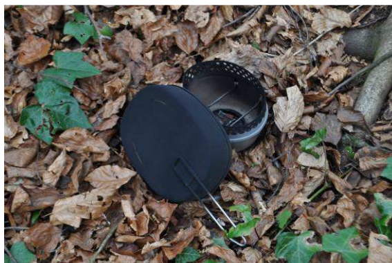
Methyl Esters competitor – Cup base after burning 1 block of fuel
