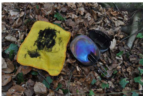
Methyl Esters competitor – Soot removed from base of cooker after burning 1 block of fuel.
