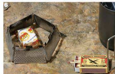
5: The new Zip tablets look similar to hexamine - to the left of the tablet is a Boilex All-In-One emergency aircrew stove and to the right is the Boilex Hinged Stove
