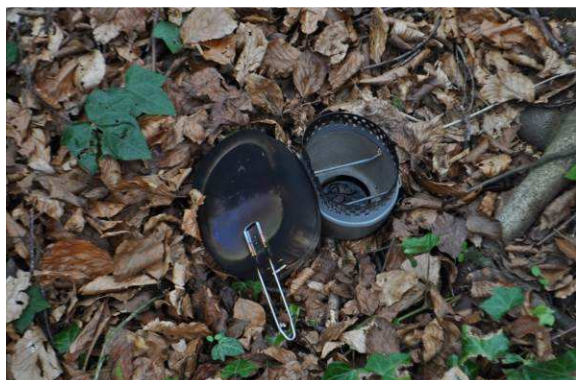
FireDragon – Cup base after burning 1 block of fuel
